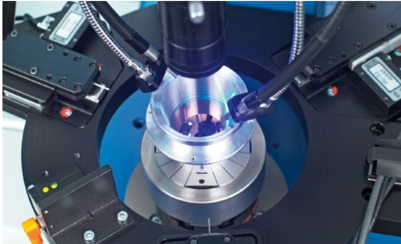
Fig. 5 Bonding station with three actuators for alignment in two degrees of freedom.
