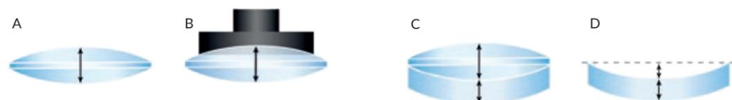
OptiSurf® LTM enables the measurement of single lenses without (A) and with (B) arbors, doublets (C) and the sag value (D).
