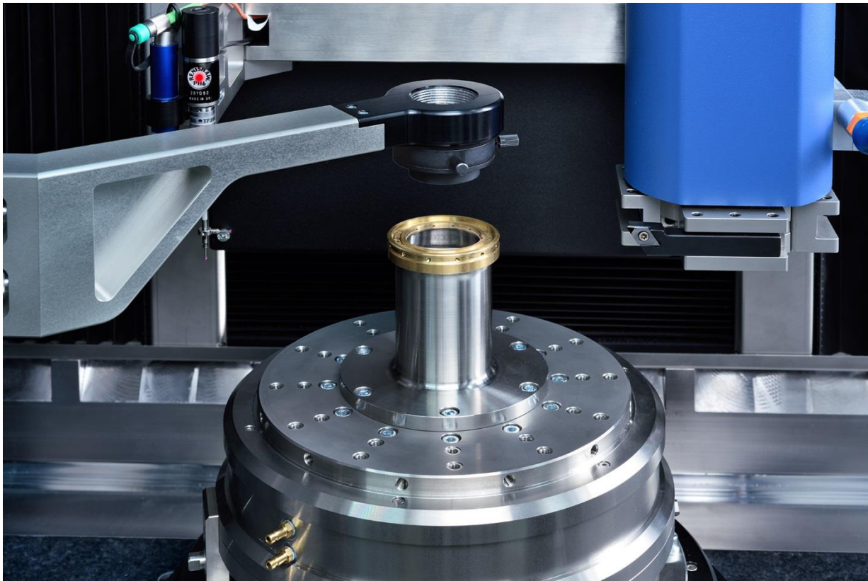
Figure 2: Measurement technology integrated in the alignment turning machine, here: integrated centering measurement technology on the basis of an OptiCentric system for determining the optical axis of the lens. Additional integrated measurement technology: Sensors for contact free distance measurement, low-coherence interferometer for determining the center thicknesses, probe for diameter determination. The entire measurement technology is integrated in the software
