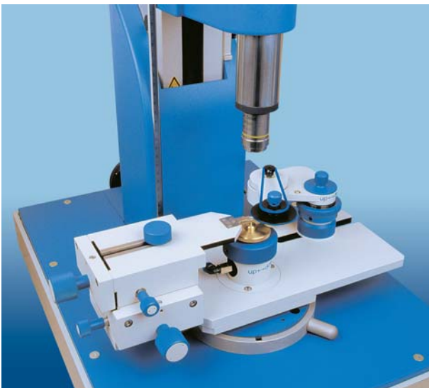
Vacuum Rotary Chuck for Centration measurement
