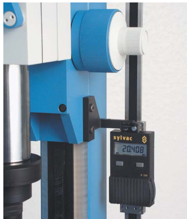
OptiSpheric® with Digital Linear Scale
